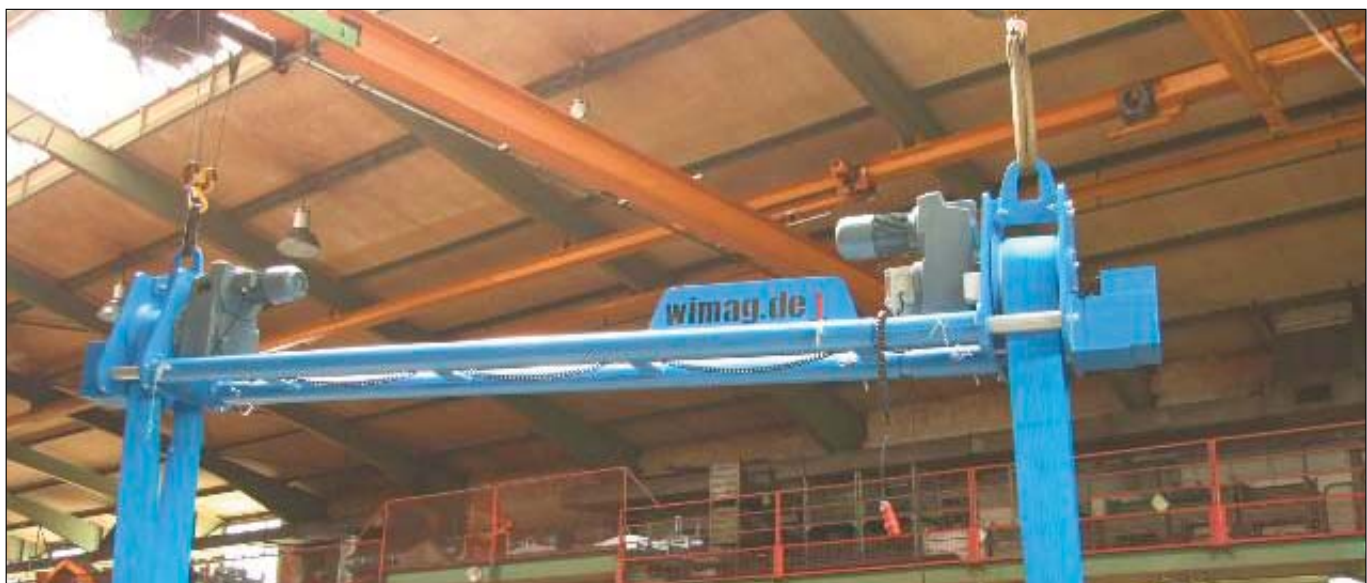
Special Design WG 7,5, carrying capacity 7,500 kg
